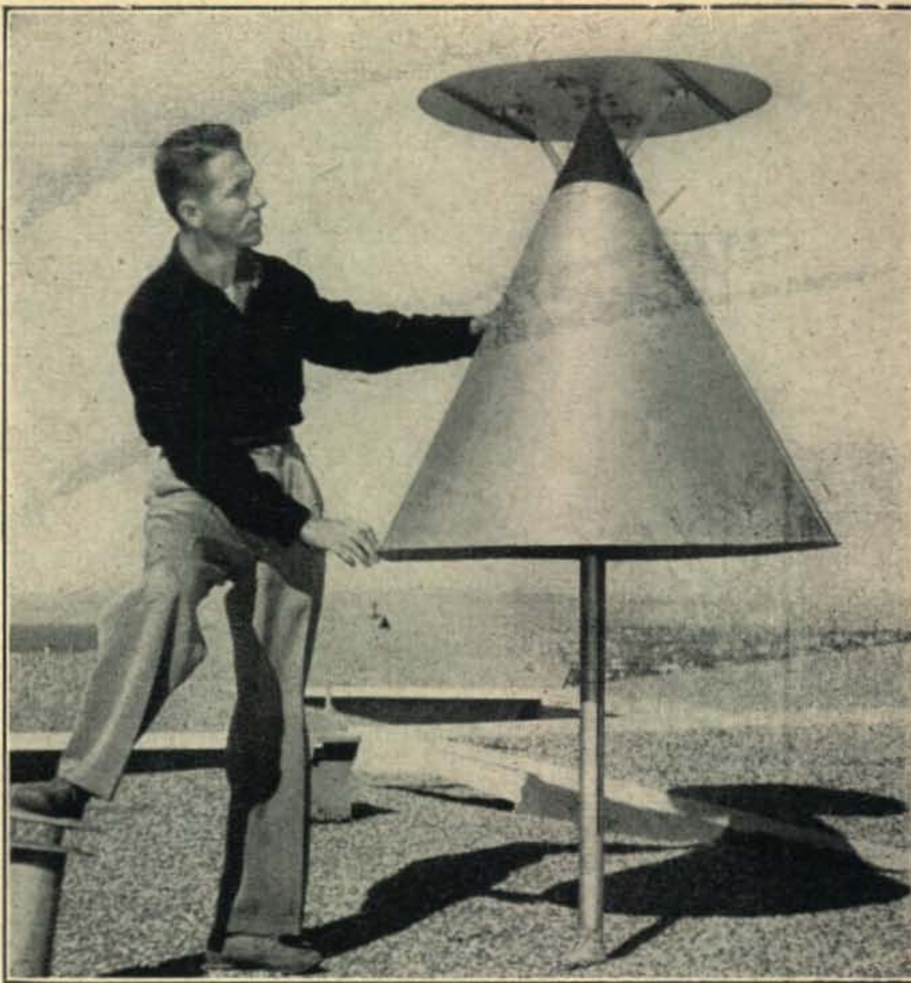
Fig. 1. W6UYH inspects a vertically polarized temporary test installation of the 40 to 500-mc discone.
